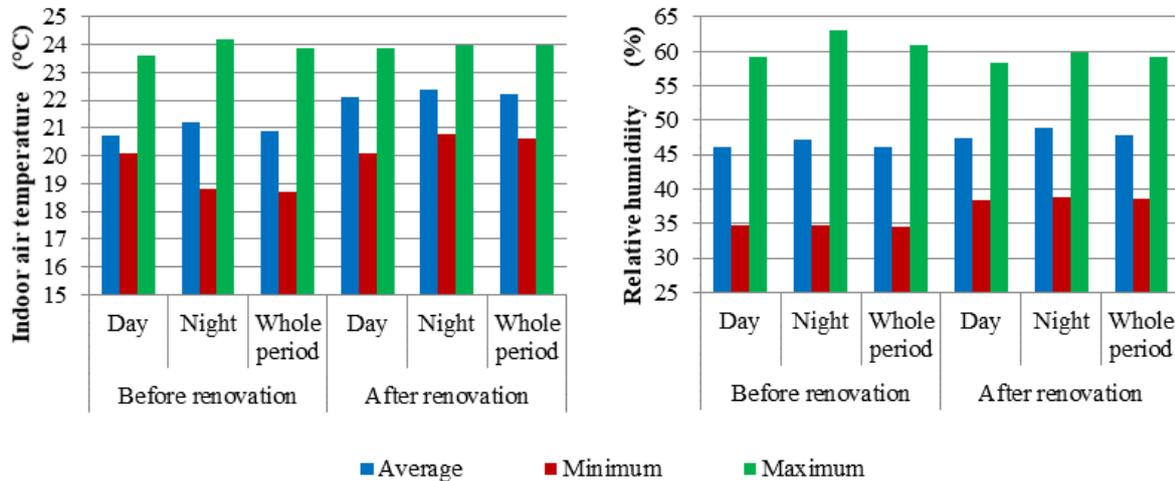
Fig. 4. Average temperatures (left) and relative humidity (right) in the apartments before and after complex renovation [16]
