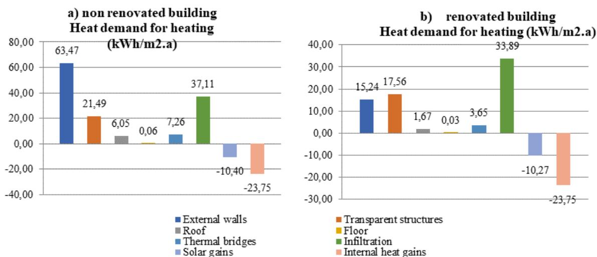
Fig. 3. Heat demand of the building (a- non renovated, b-renovated)
