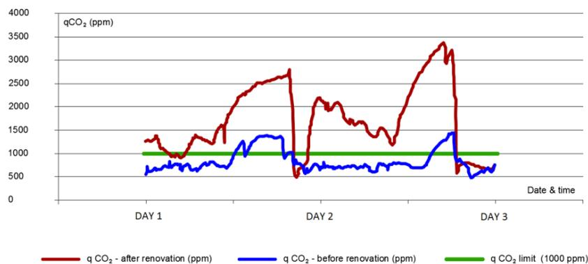
Figure 5. Example of CO<sub>2</sub> concentration in one selected apartment during two days out of the whole measurement period before and after the renovation. [15] [16]
