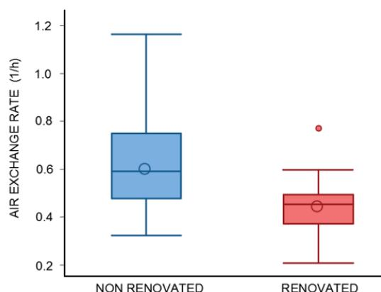
Figure 7. Air exchange rate before and after renovation as a statistical output [15] [16]
