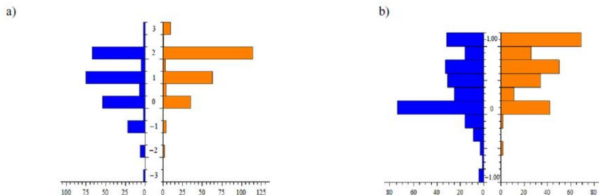
Figure. 2. Thermal sensation (a) and acceptability of thermal environment (b) evaluated by occupants of original (blue bars) and retrofitted (orange bars) residential buildings.
