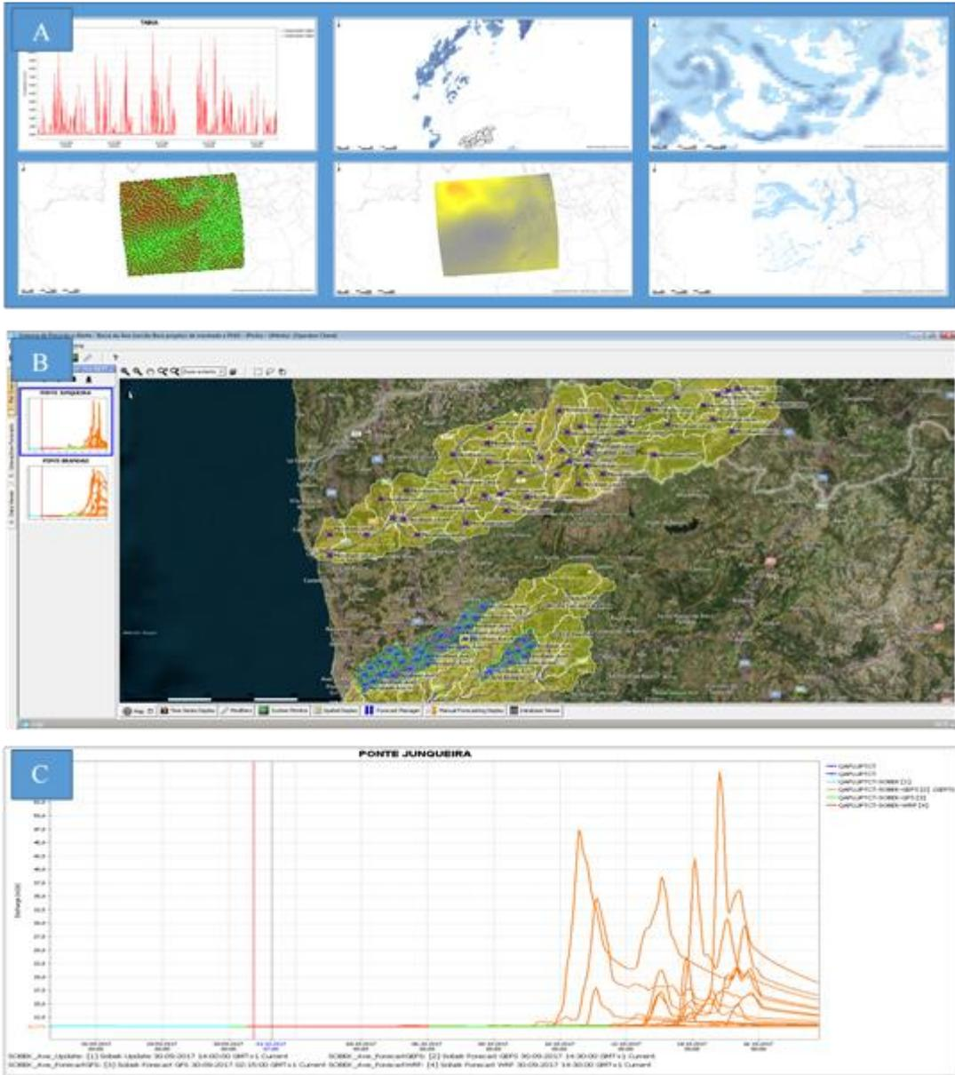
**Figure 1** Flood forecasting system for the NW Portuguese region. A) historical and forecasted data, B) hydrological sub-basins for river Lima and river Ave basins, and C) predicted river Ave flow rates at Ponte de Junqueira.
